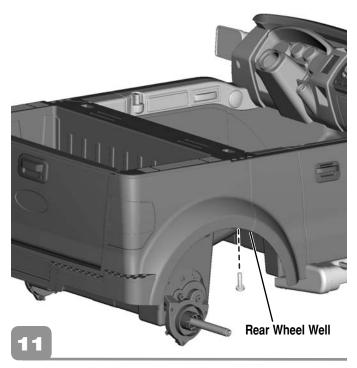
• Insert a screw up through both rear wheel wells and into the cargo bed. Tighten the screws.
